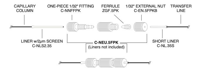
As the diagram illustrates, liners allow standard nanovolume fittings to hold capillary tubing. The short liner (product number C-NL.35S) is used with the external fitting, while the long liner (product number C-NLS2.35) is used with the internal fitting. The liners are designed for tubing with an outer diameter of 340-360  $\mu$ m (~0.35 mm). Call us about the availability of liners for other sizes of tubing.
