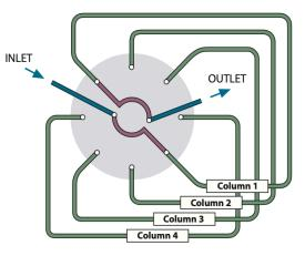
actually requires an actuator programmed for eight positions, with position 5 selecting the same column as position 1, 6 the same as 2, etc. A six column valve needs a twelve position actuator, with 7 the same as 1, 8 the same as 2, etc.
