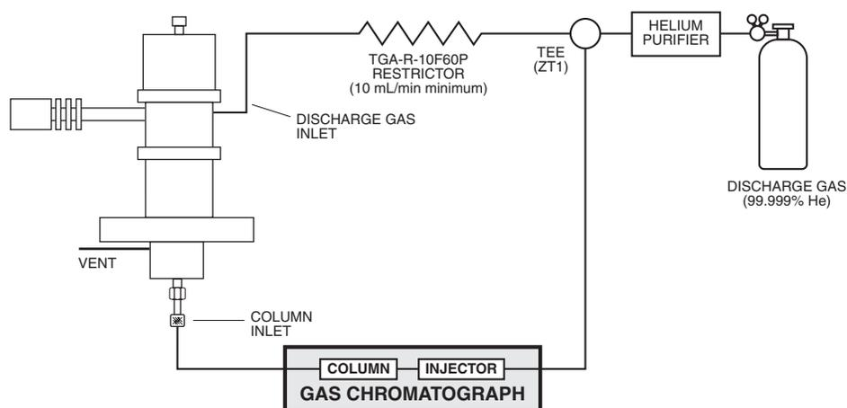
**Figure 3:** Gas connections for a PD-D2-IM system
