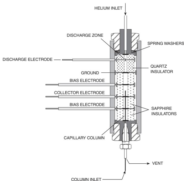
**Figure 1:** Schematic of the D-2-IM detector
