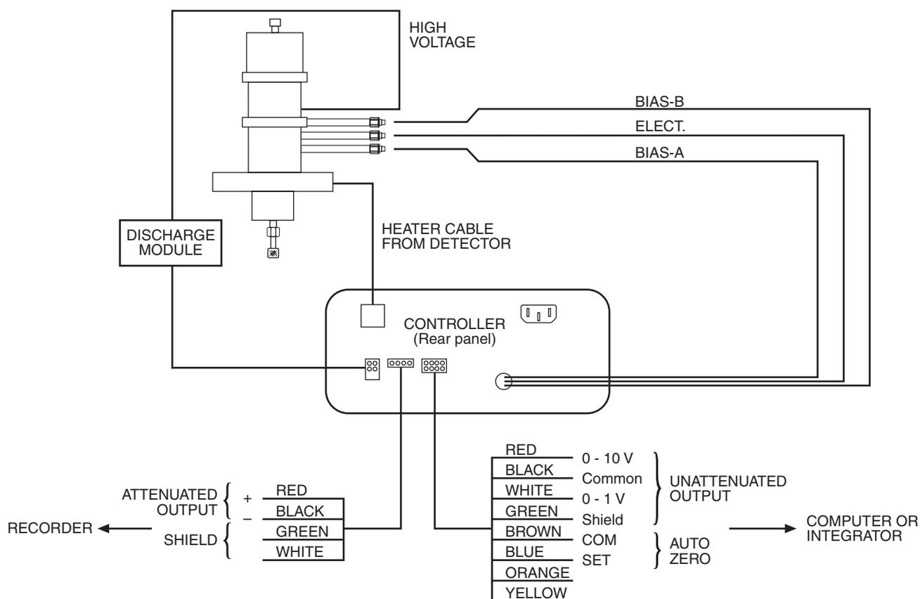
**Figure 4:** Electrical connections
