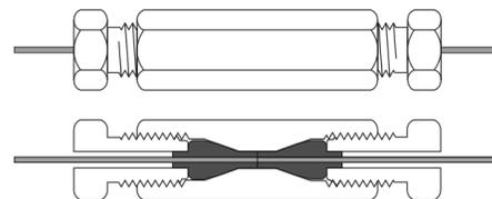
Valco one-piece adapters differ from standard ferrules by the addition of special “nibs” on either end. The nib on the back of the ferrule prevents misalignment and cold flow problems. The front nib fills the pilot volume, eliminating dead volume and insuring alignment with the other tubing or with the through bore of the union.
