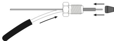
4. Slide the ferrule over the liner, using the installation tool to keep the liner all the way into the nut.
