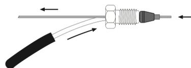
5. While continuing to hold the liner in place with the tool, pull the fused silica tube back until its end is flush with the liner.
