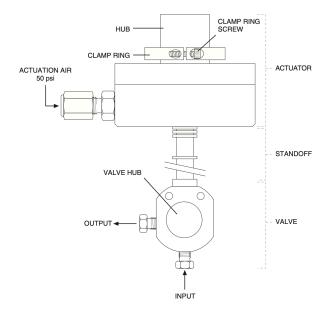
3. 1/16" versions ONLY: Mount with the two holes located in the valve body itself. There is clearance for #6 screws.
